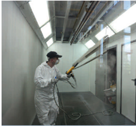
The air flow is guided in a vertical direction, which allows the application of two colours per lifting beam.
