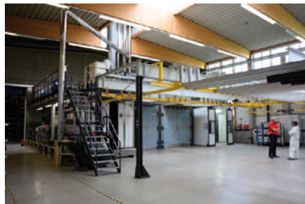
An overview of the plant, from the left to the right: pre-treatment, adhesive water dryer, enamelling furnace, powder-coating booth. The intermediate floor accommodates the components of the pre-treatment and exhaust-air systems.
