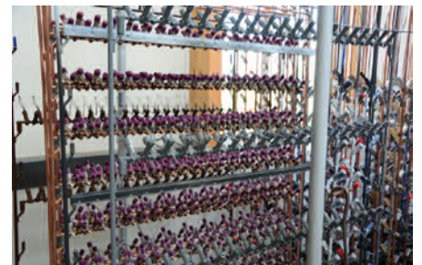
For the handling of profiles, faceplates and fasteners, a variety of product carriers are available, which can be suspended from the lifting beams.
